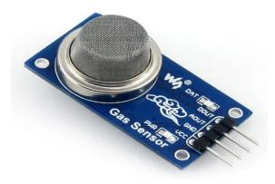
MQ-135 Module sensor has lower conductivity in clean air. When the target combustible gas exist, the sensors conductivity is morehigher along with the gas concentration rising. Convert change of conductivity to correspond output signal of gas concentration. MQ135 gas sensor has high sensitivity to Ammonia, Sulphide and Benzene steam, also sensitive to smoke and other harmful gases. It is with low cost and suitable for different applications such as harmful gases/smoke detection.
